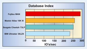
It is in IOMeter that the MAN3367 gets to flex its muscles. The drive's File Server Index bests the Atlas10k III by over 9%. The margin is much narrower in the Workstation Index...nonetheless, the Fujitsu drive stays on top by about 3%. The MAN's lead grows back to 9% in the Database Index. With the Cheetah 73LP trailing the Atlas in all three IOMeter categories, it does not even enter the equation.
